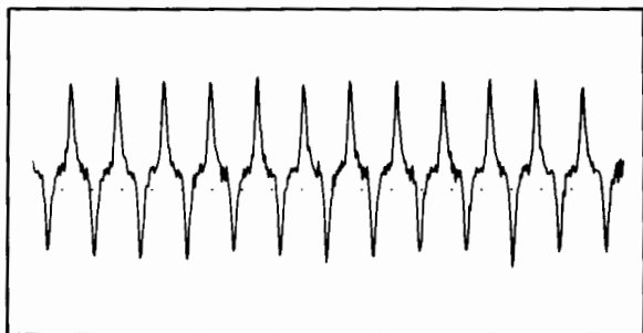
This signal was recorded from a floppy disk read head.
