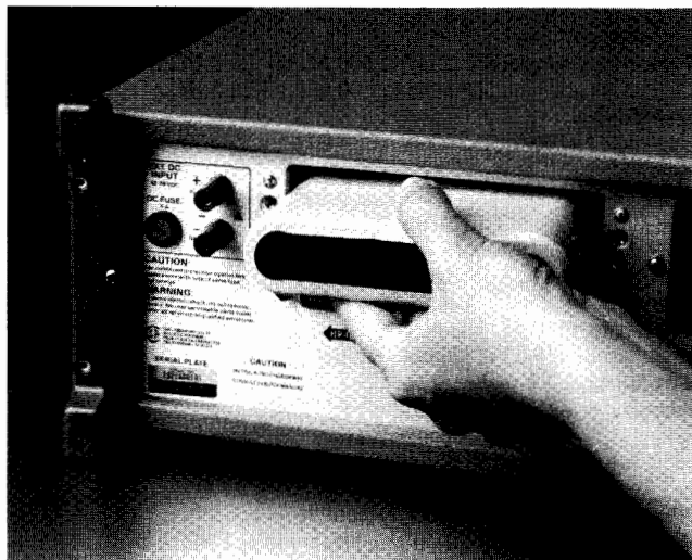
The internal battery allows measurements without cumbersome electrical cords.
