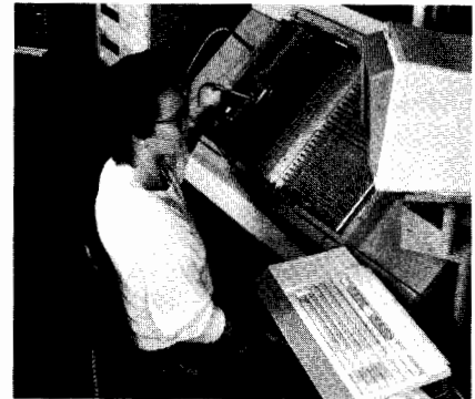
HP 3070 board test systems locate faults and faulty components on PC boards.
