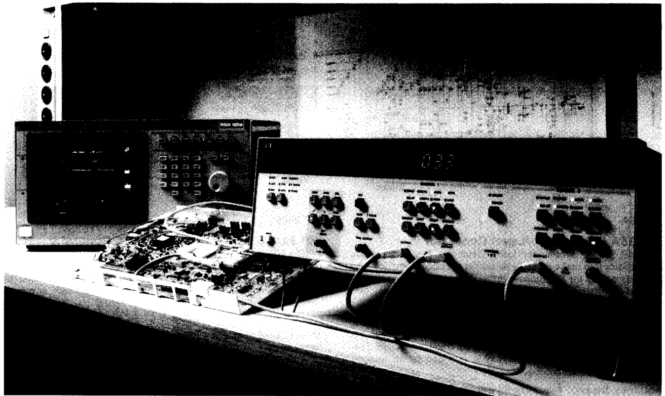
Typical stimulus-response test setup. The HP 8131A pulse generator in the foreground generates 500 MHz pulses with typically 120 ps transitions (20 to 80% of amplitude). The HP 54120 series oscilloscope measures device response.
